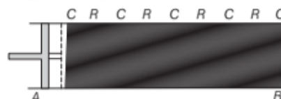
Production of Longitudinal waves in a cylinder by moving a piston back and forth.
